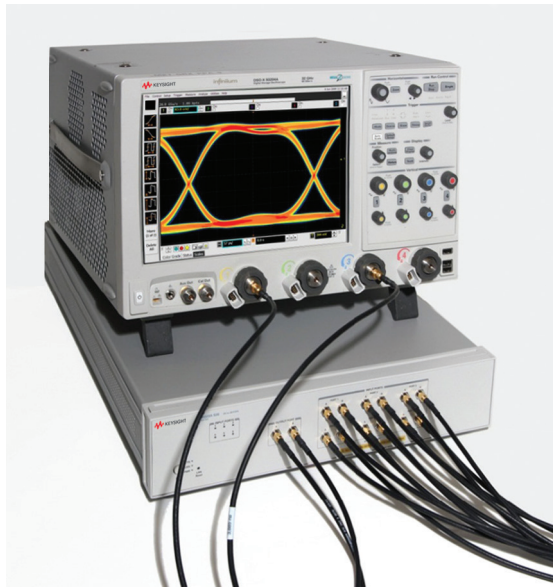
Figure 14. Automated testing for multi-lane digital bus interface through switch matrix.
